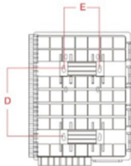
Pic 2 Installation Size
